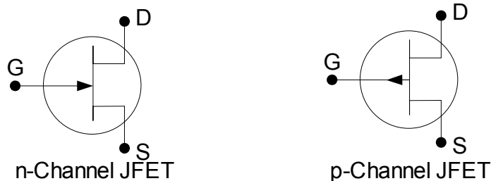
Drawing 17: Schematic Symbols for J-FETs
