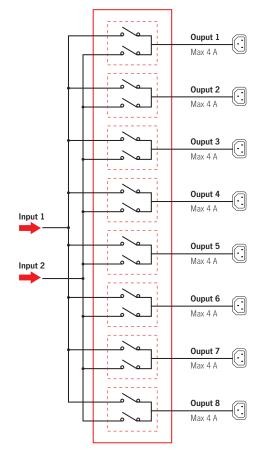
**Multi-SWITCH** improves electrical supply continuity. The principle of operation guarantees a higher reliability level than that achieved using a single UPS (on-line with automatic bypass) or several UPS in parallel.
